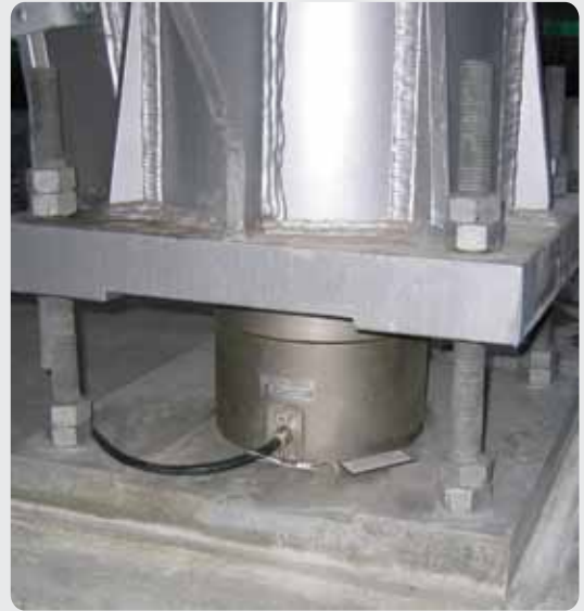
▲ Installation of compression load cells requiring lift-off protection
